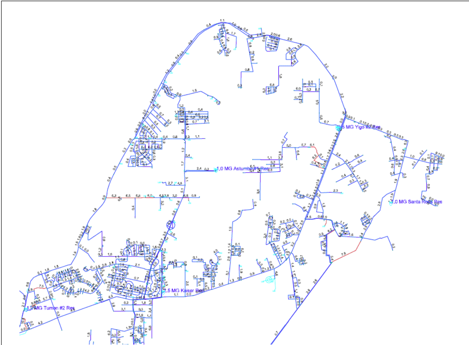
Figure 6-12 - North System 1, Max-Day, Max Velocity (>6 fps)
